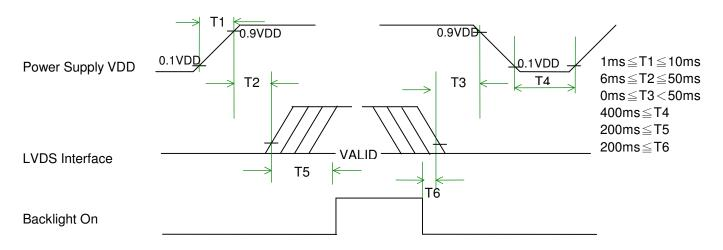
Apply the lamp voltage within the LCD operating range. When the backlight turns on before the LCD operation or the LCD turns off before the backlight turns off, the display may momentarily become abnormal.
